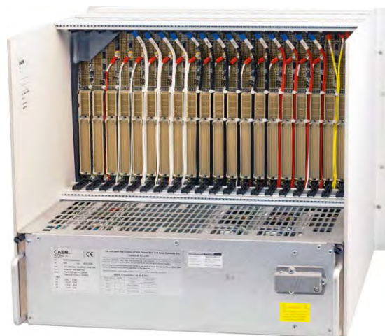
VME8200 shows a full accessible rear side of its VME64X backplane and a full sized rear side card cage for 3U/6U x 80mm transition modules.
