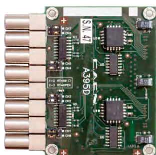
A395D 8 NIM/TTL input/output channels
