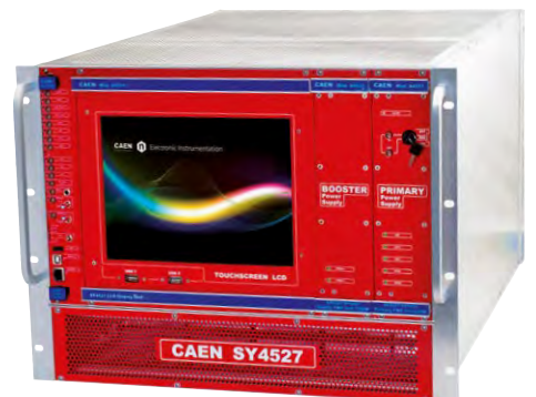
SY4527 Full with LDC monitor front view
