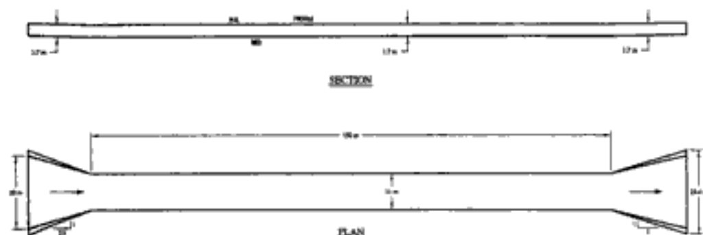
Figure 5-1. Channel contraction and expansion
