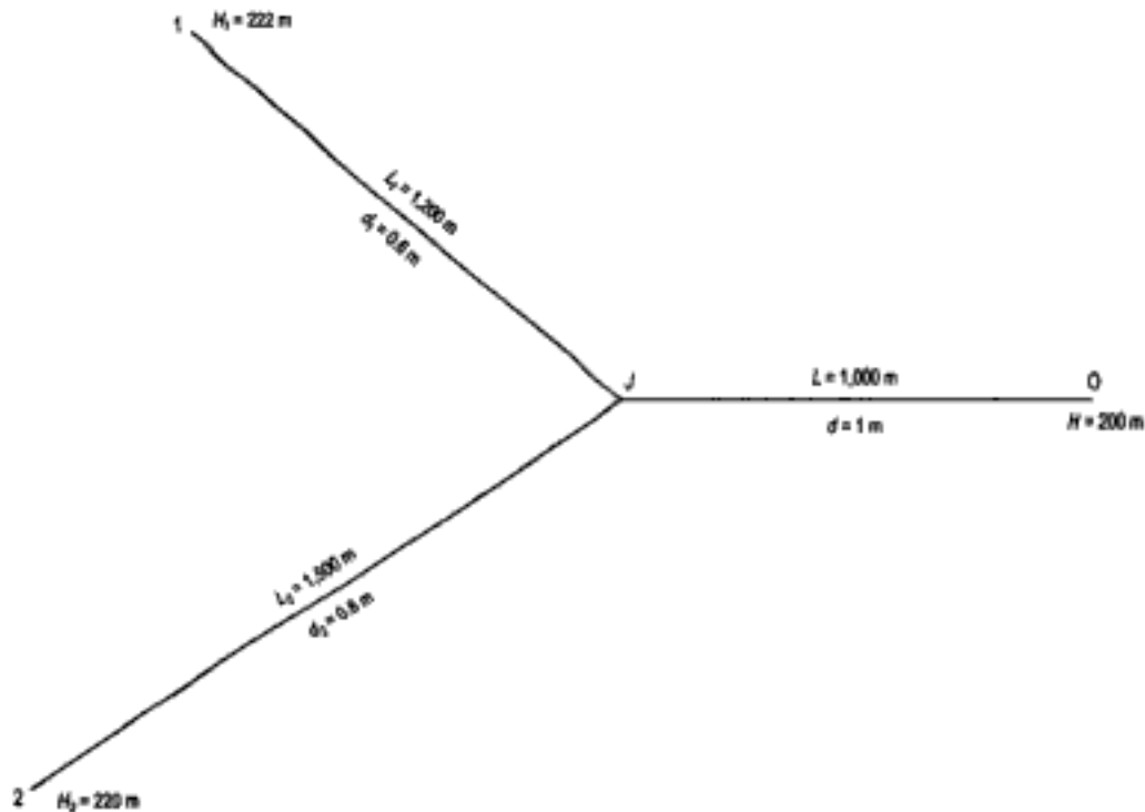
Figure 3-10. Schematic of water supply lines
